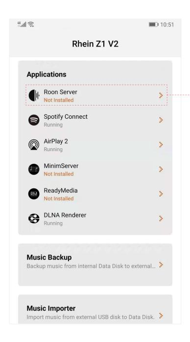
In the Applications section of main page, check the status of Roon Server. If the status is "Not Installed", you will need to install Roon Server to this Z1. Click on ">" to enter the Roon Server page.
