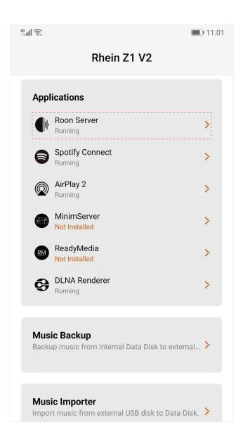
Be noted to configure the Audio Selector to choose Roon Server as Audio Source. Click on "Change" and choose Roon Server to make Roon Server to use the USB DAC connected to this Z1.
